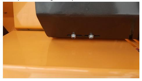
This adjustable plate hits the return bar to put the ram into neutral.
