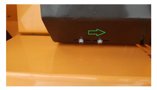
Tighten both nuts and try the ram function, the ram should now return to home properly but the ram should not be all the way into the processor housing. What you need to do is adjust the back ½" to the left, tighten the nuts and try the ram function again, keep trying this until the ram stops properly and the ram housing is either flush or protruding no more than ½" out of the processor housing.
