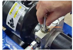
6) When you pull the housing out you will see the stainless steel screen that needs cleaned, use brake cleaner or degreaser and a brush to clean the screen out. Screen can be removed if necessary for cleaning.
