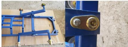
6.) Install all 4 tires, R's on one side, L's on the other and tighten wheel nuts to 40ft/lbs.
