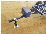
11.) Slide the swivel coupler mount in, position the swivel up or down depending on your ATV hitch height, tighten both bolts.
