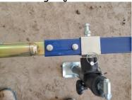
14.) Install hydraulic fitting into cylinder, install brackets and cylinder on frame, tighten all 4 bolts.
