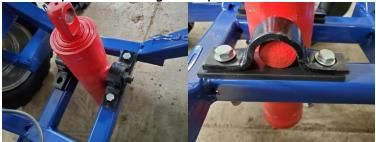
15.) Install hydraulic pump-there are two short, gold colored bolts that came in the same box as the hydraulic pump unit.
