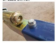
13.) Slide tongue jack to desired position, usually about 15cm (6") back of 1st swivel coupler bolt.
