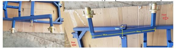
4.) Install 13mm bolt & nut washer through the plate on the pin and the frame tab, tighten nut & Bolt. Install cotter pin, repeat for the opposite side.
