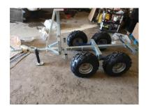
12.) Find the orange 45° brackets and slide into the cavities on each frame end.
