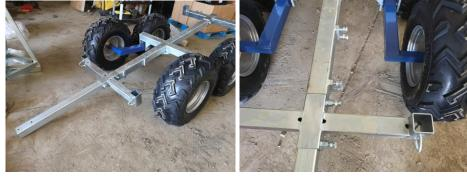
8.) Slide the cage over the inner frame rail. Installed right up against front frame portion. Install 2 large bolts and tighten.
