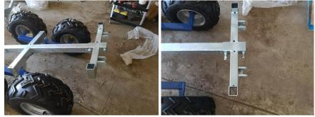
7.) Slide the front frame portion over the main frame. Slide it right up to the main frame. Install 2 bolts and tighten.
