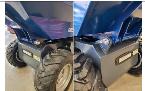
Flip up the bucket and extend cylinder to help with installing the next pin
