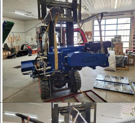
Straps need to be placed on the outside of the engine and hydraulic tank as shown in pictures
