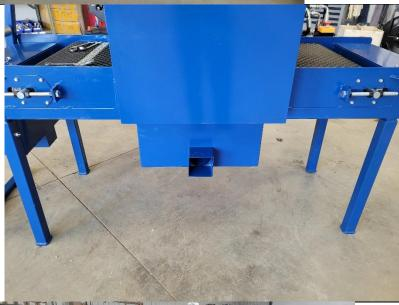
Table with rollers can now be attached, leaving the three bolts loose for now
