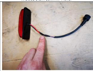
Remove the black tape as shown in the photo above and separate the wires as shown in this photo
