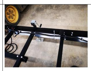
A photo showing a harness bracket near the rear of the trailer
