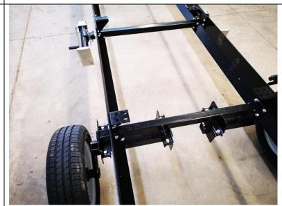
Next, you will be installing the rear end plate onto the trailer
