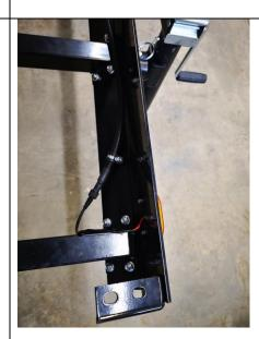
A photo of the wiring slack at the rear of the trailer
