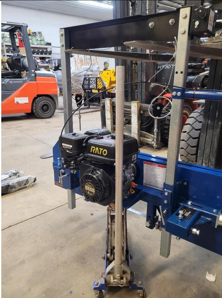
Attach push handle to the post on the lower two of the four holes.
