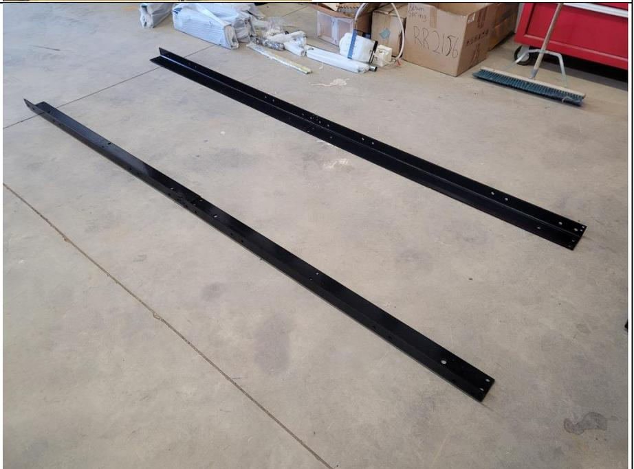
Attach the two sections of rails of each side together using the track alignment bracket with four holes
