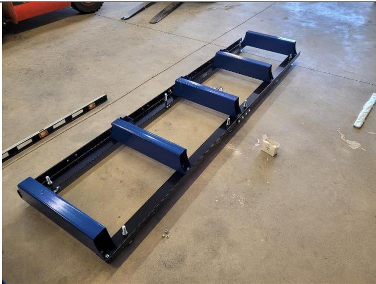
Before lifting the carriage onto the rails make sure to install the carriage stops
