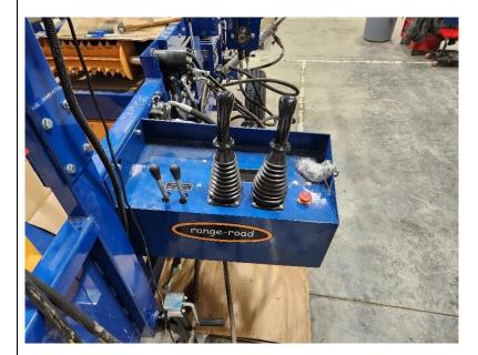
To operate the splitting ram; pull BOTH of these levers down at the same time. When the ram reaches the end of its stroke, the left "splitter" handle will kick off automatically. The ram will then return automatically and once it is fully retracted, the right "return" lever will autmatically kick off. This will put both levers back into the center, neutral position.
