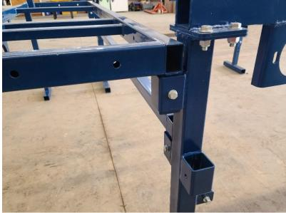
Now the support beams will be installed between the legs.
