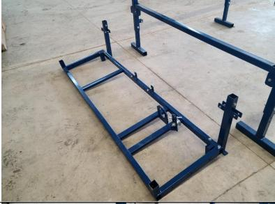
Ensure the tabs on the intermediate legs are facing lengthwise down the infeed, as shown here.
