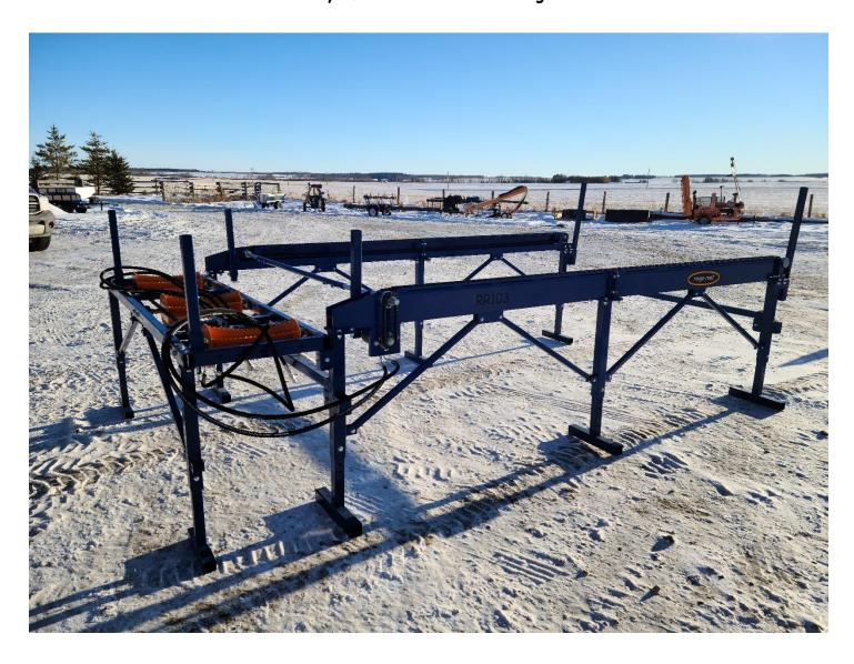
This table is designed to be used on either side of the processor and this table has an extension kit available to add an extra 7' of width -The RR104
