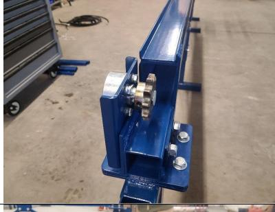
When installing the chain adjustment plates, run the long, tensioner bolt "in" to allow the adjustment gear to be as close to the rails as possible.
