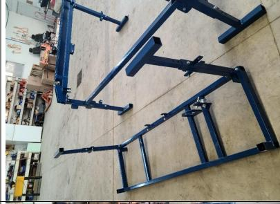
With assistance, flip the infeed over and into the square brackets on the table.
