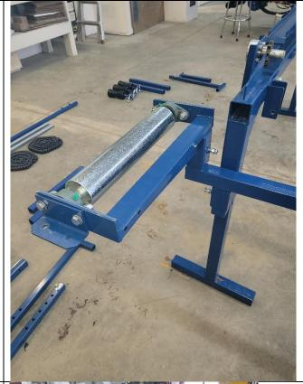
Attach the three support legs to the infeed section of the table.
