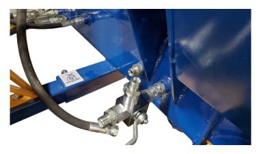
The hose you uninstalled will be connected to the fitting in the middle of the valve assembly.
