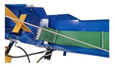
Crank up the conveyor almost all the way. Watch that the belt is not sliding of the conveyor.
