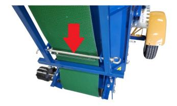
Use those 2 safety pins to lock the conveyor to the frame.
