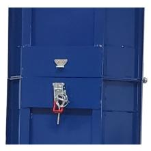
Move this bar so that it is across the belt and in the catch on the conveyor.
