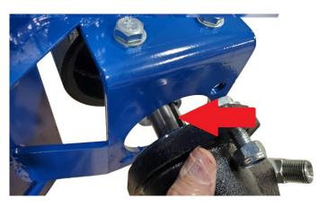
Install the motor and watch for the key to be in the key way.
