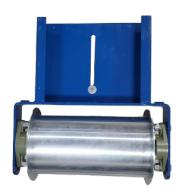
Slide this into the conveyor end. Install the bolt and tighten but leave it loose enough so it can move.
