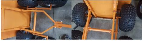
12.) Mount winch post and support to front of hitch arm, do not tighten bolts.
