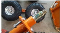
4.) Insert axle into walking beams.
