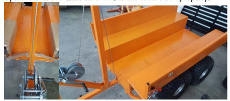
19.) Install doors inserting pins into pipes on trailer.
