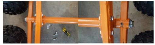
7.) Mount subframe to axle, do not tighten bolts.
