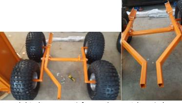
8.) Attach hitch arm to subframe, do not tighten bolts.
