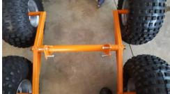
5.) Install washer, retainer and aluminum nuts to hold walking beams onto axle. Leave the nut loose enough that walking beam can move freely, bend tab into nut to lock in place.
