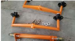
2.) Mount the wheels to the walking beams, tighten nuts.
