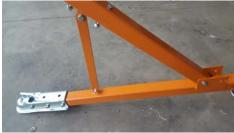
13.) Install winch pulley shaft. Tighten bolts for winch post and 2" coupler, bolt for winch pulley post is to be snugged up but post must be able to move.
