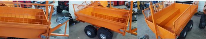
22.) Line up pins and install front & rear mesh sides.
