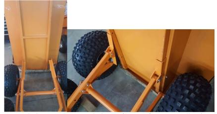
11.) Line up holes on mounts to holes in frame of box, install bolts & nuts, tighten all subframe bolts.
