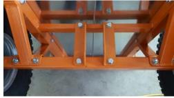
8.) Put hitch arm into place, install nut & bolt, tighten nut until bolt sits in plastic lock, tighten bolts on pivot brackets.
