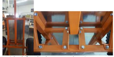
9.) Lock latch from hitch arm to trailer tub.
