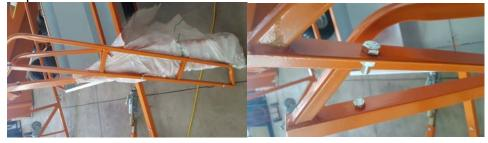
19.) Mount side rails and tighten bolts.
