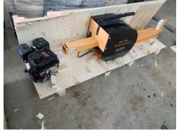
3.) Lift the main splitter frame and bolt on engine mount frame. The main frame is very heavy and should be lifted with an engine hoist or something similar that can support the weight and keep it stable. If lifting only one end at a time make sure that the unit is stabilized and cannot slide or fall.
