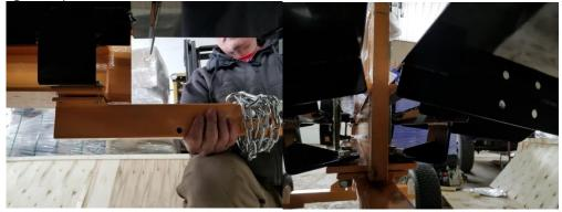
10.) Install the 2 angle brackets to bottom side of log tables, snug all 8 bolts up, ensure that top of the log table are even with sides butting up to each other, not overlapping or un even, tighten all 8 bolts.
