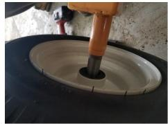
5.) Snug the nut up and insert cotter pin and hub cap, the nut does not need to be torqued because these are low speed turf tires. Repeat for the other side.
