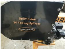
17.) Mount cover and tighten all the bolts including the angle bracket on bottom.
