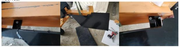
9.) Mount the hitch tube to the front four bolts used for the log table mounting, snug bolts up but do not tighten yet.
