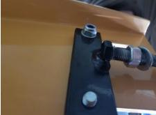
14.) Adjust the tensioning bolt below engine until belt is snug, there should be approximately  $\frac{1}{2}$ " of movement, secure backnut to lock in place. Snug up engine mount bolts.
