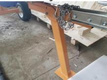
13.) Lower engine into place inserting V-belt into engine pulley, mount engine with the 4 supplied bolts, outer bolts must go through the adjustment plate underneath plate, do not tighten bolts.
