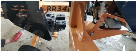
18.) Fill engine with oil as specified in manual.
