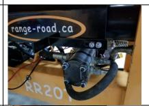
The front bracket hits the post on the manual return arm as the ram returns home, this must hit the post before the ram hits its internal stops, softening the stop.
