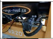
The front bracket hits the post on the manual return arm as the ram returns home, this must hit the post before the ram hits its internal stops, softening the stop.
