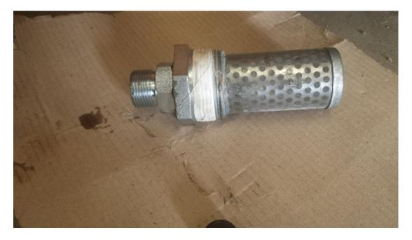
If processor does not have a magnet on the drain plug it is advisable to install one either in the tank or on the drain plug as pictured, put new thread tape on drain plug and re-install until tight
