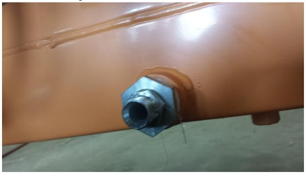
Clean out any dirt or debris in bottom of tank, if possible flush tank with 2-3 litres of clean Hyd. Oil
